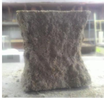
Figure 3.4 Failure pattern of cube samples after compression test
