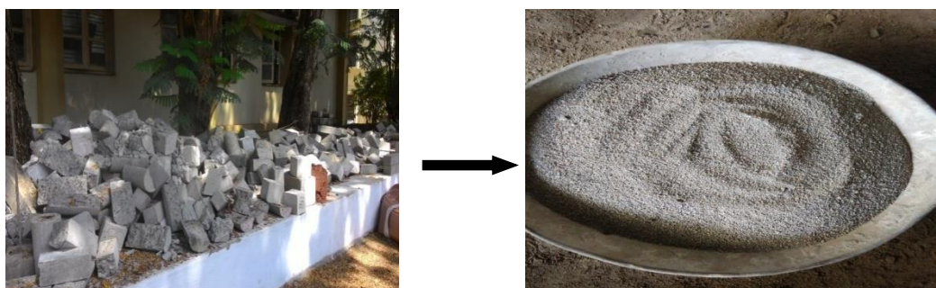
Figure 3.1 Formation of RFA from tested concrete Specimens
