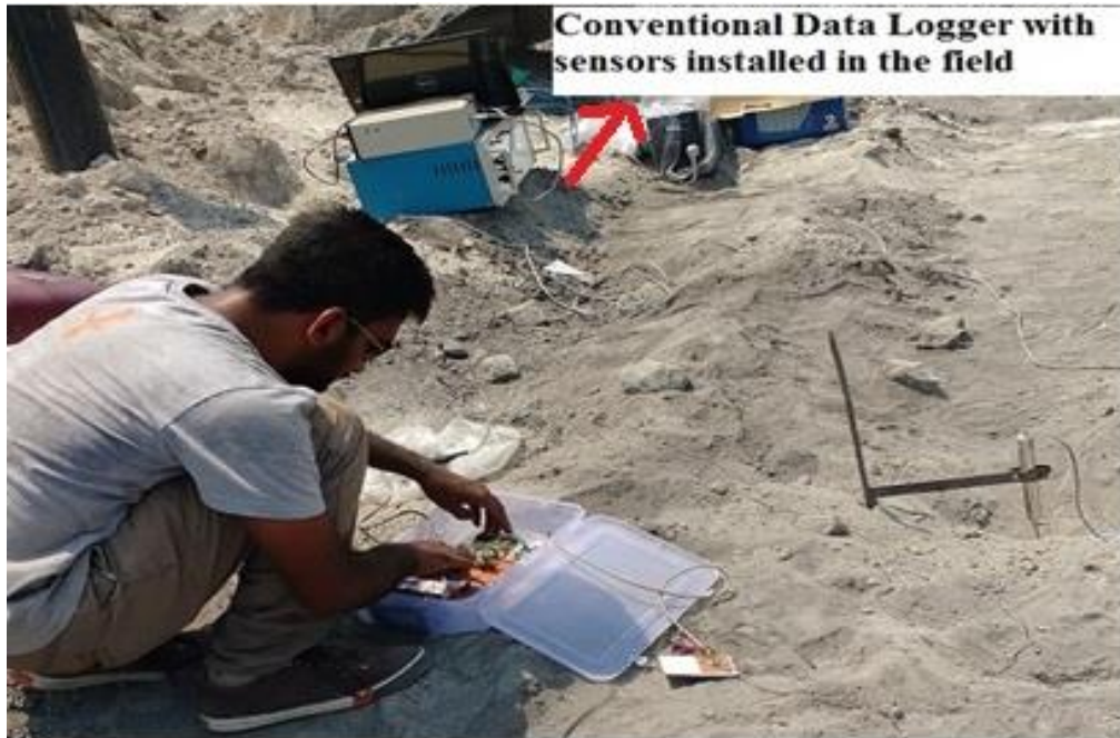
Fig. 3.24 Connection of sensors to the data logger in the field
