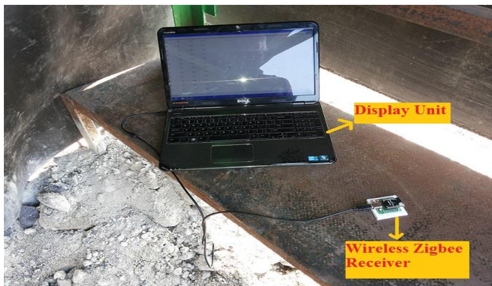
Fig. 3.19 A view of base station in the field
