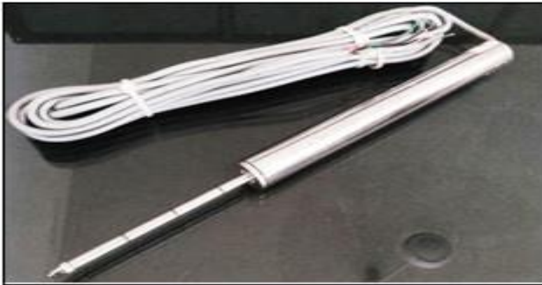
Fig. 3.2 A view of AC LVDT being used in the field
