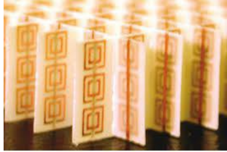
Figure 2.4: An MTM media made of SRR and copper strips
