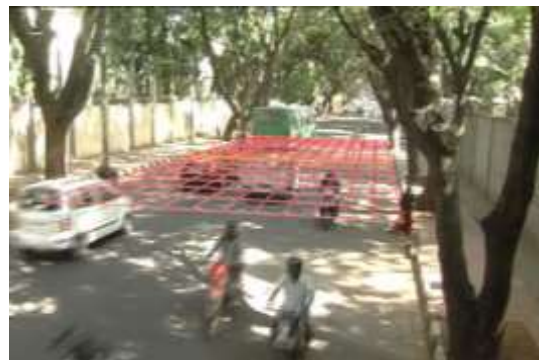
(b) Gridlines for longitudinal and lateral gaps
