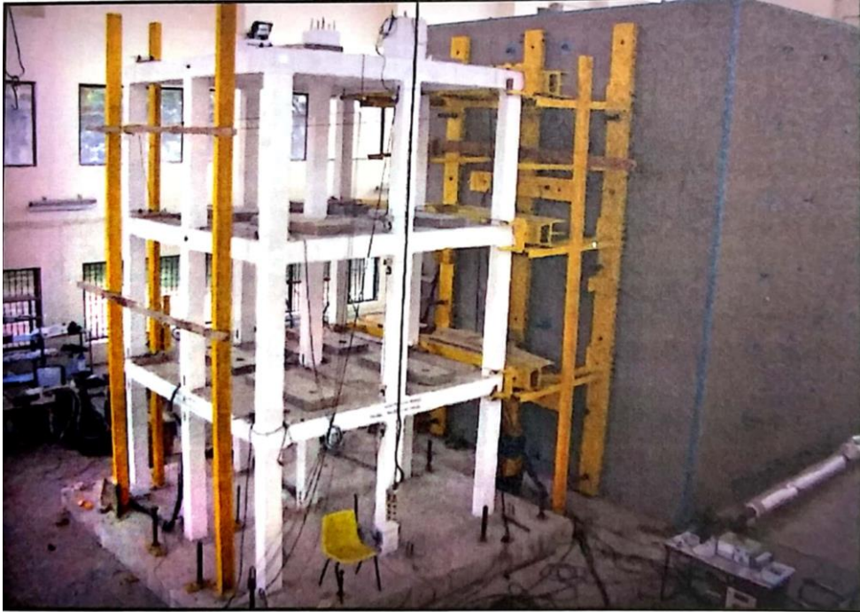
Fig. 5.1(a). Experimental setup for pushover analysis
