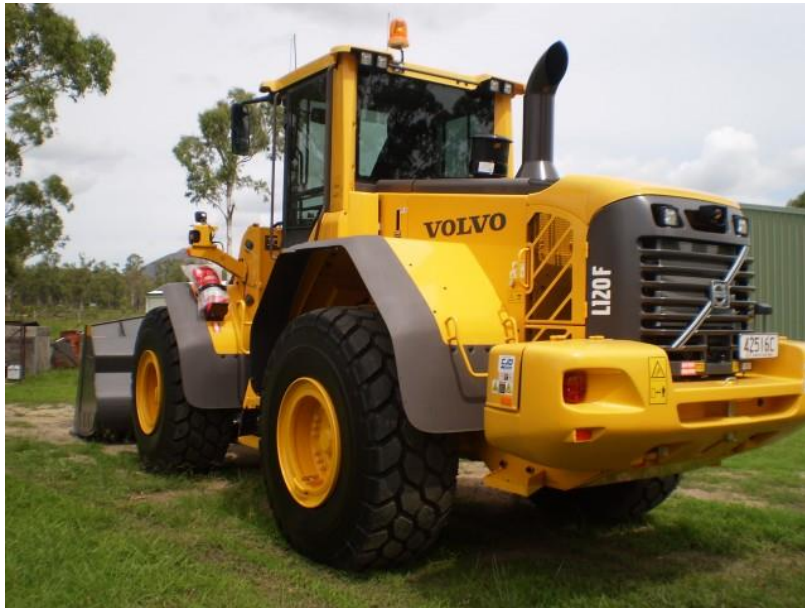
Fig. 9.2 Volvo wheel loader, Model: L120F
