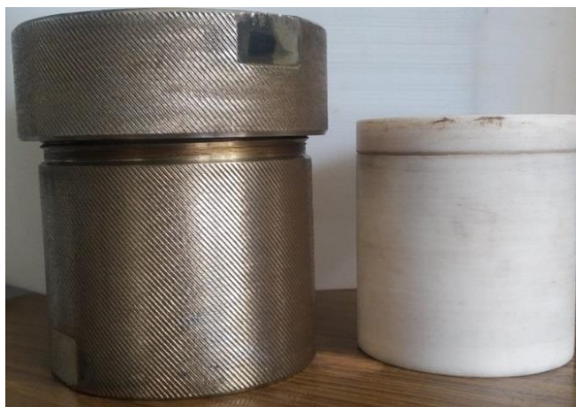
Figure 2.1 Stainless steel jacket and teflon jar of a hydrothermal setup.
