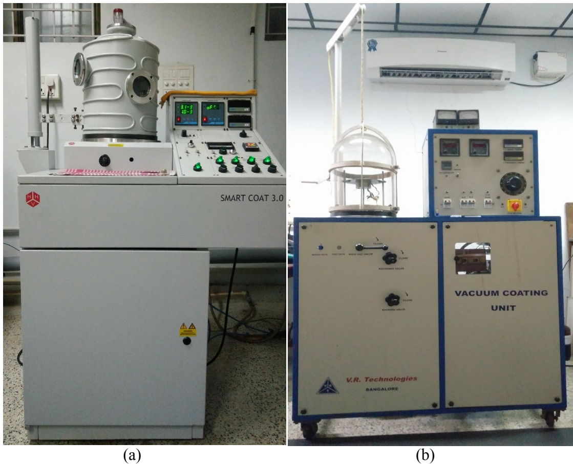
Figure 2.2 Photographs of thermal evaporation systems used to deposit, (a). \text{In}_2\text{Te}_3 films and (b). InTe films.
