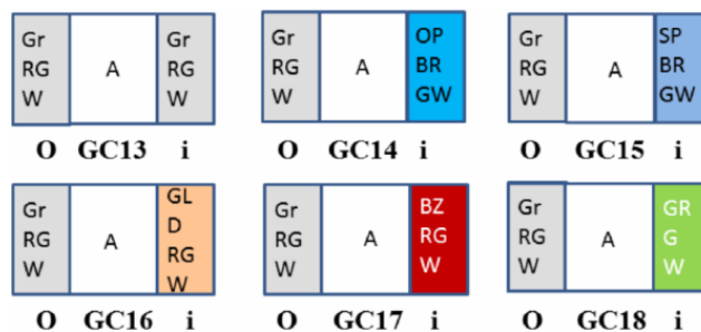
Figure 5.4.15 Grey reflective glass window combinations GC13 to GC18 with an air gap of 10mm, O-Outdoor, i-Indoor
