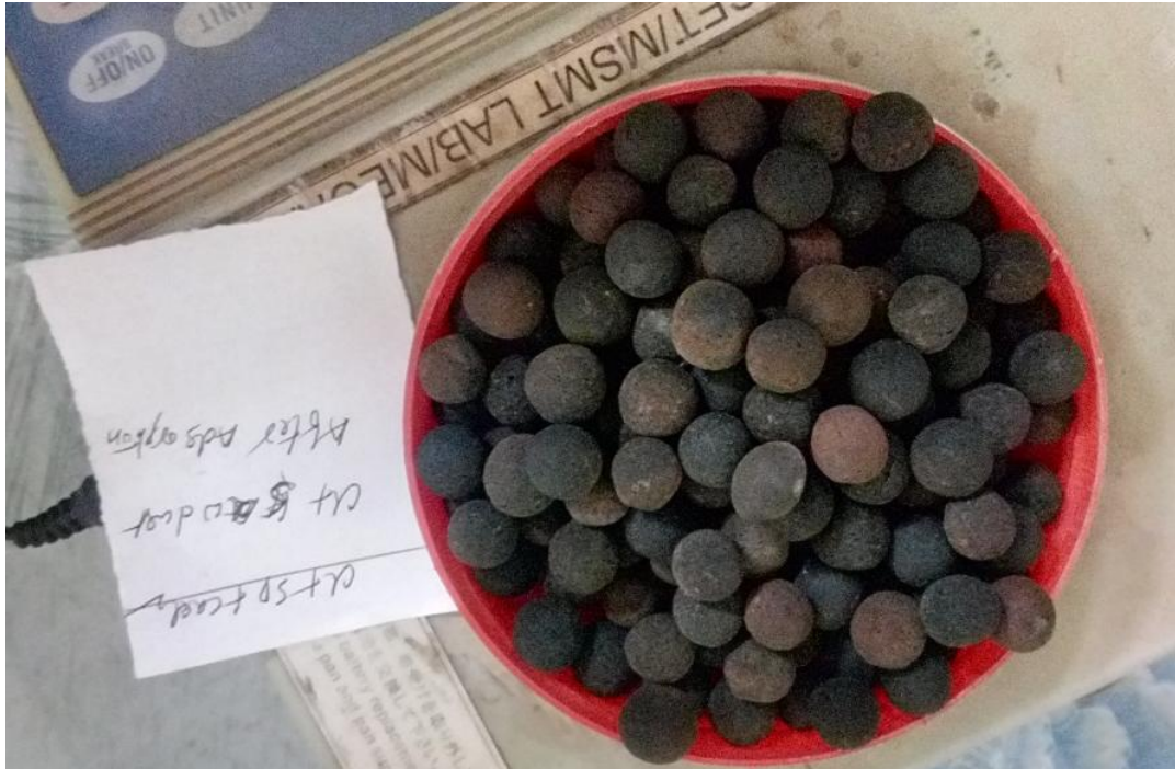
Fig. 5.16 Photograph showing the size and shapes retained by desiccants with increased use for burnt clay - sawdust - \text{CaCl}_2 .
