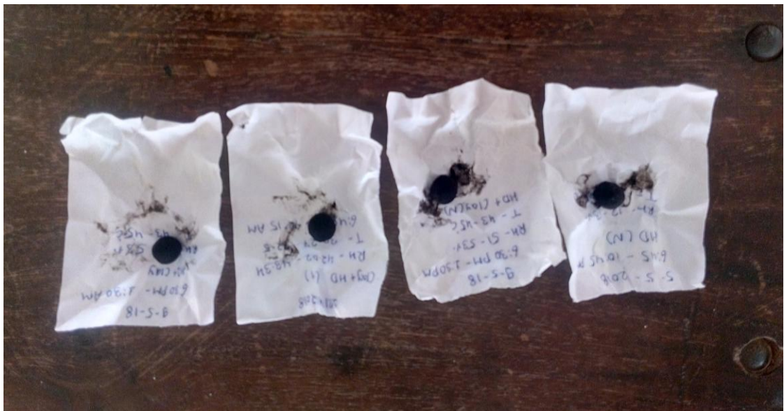
Fig. III. 6 Photographs are showing moisture uptake by heat-treated clay - 20% horse dung - 50% \text{CaCl}_2 composite desiccant.
