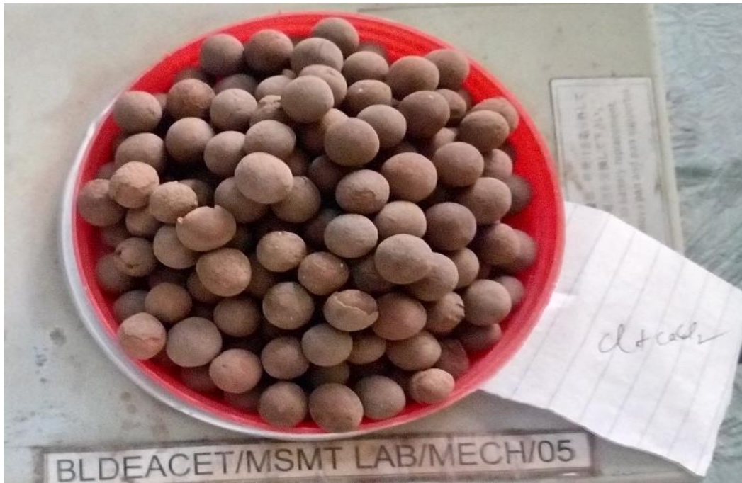
Fig.5. 14 Photograph showing the size and shapes retained by desiccants with increased use for burnt clay - \text{CaCl}_2 .
