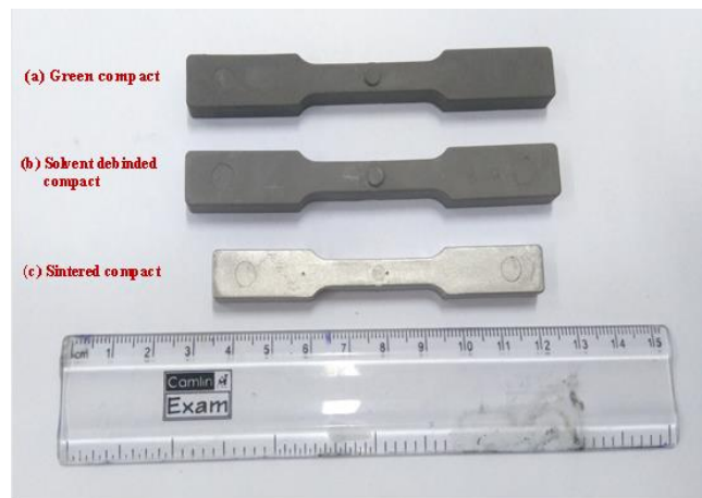
Figure 3.26 Tensile specimen sintered at 1200 °C
