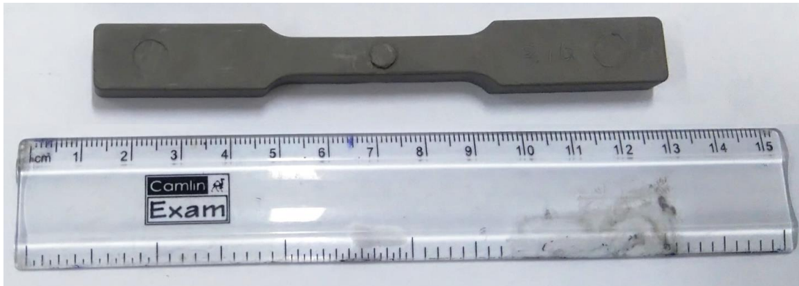
Figure 3.24 Photograph of thermal debound specimen
