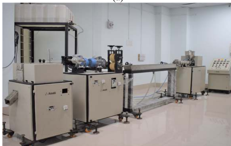
Figure 2.5 (a) Schematic representation of the industrial scale single screw extruder and (b) experimental set up.
