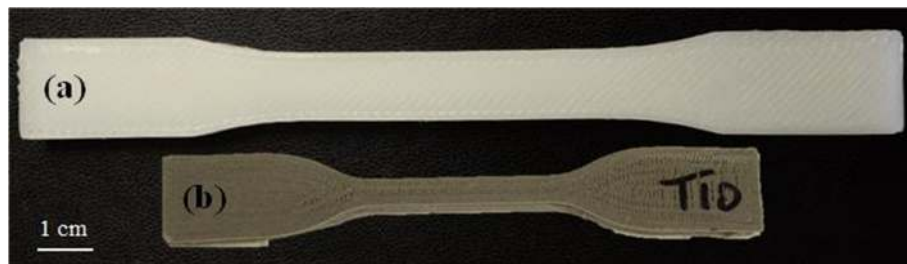
Figure 3.9 3D printed (a) HDPE and (b) H40-2X tensile bar.
