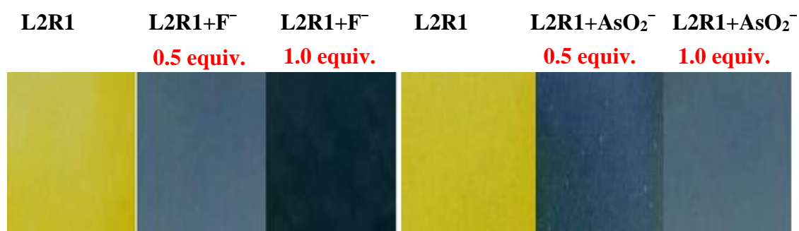
Fig. 3.59 Colour changes observed on addition of 0.5 equiv. and 1.0 equiv. of F - and AsO 2 - ions on test strip coated with L2R1 solution
