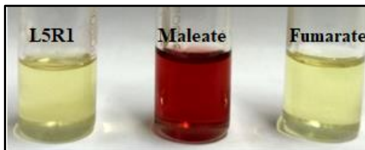
Fig. 6.42 Colour change observed upon addition of 2 equiv. of maleate ion and fumarate ion ( 1 \times 10^{-2} M in DMSO) to the receptor L5R1 solution ( 2 \times 10^{-5} M in DMSO)
