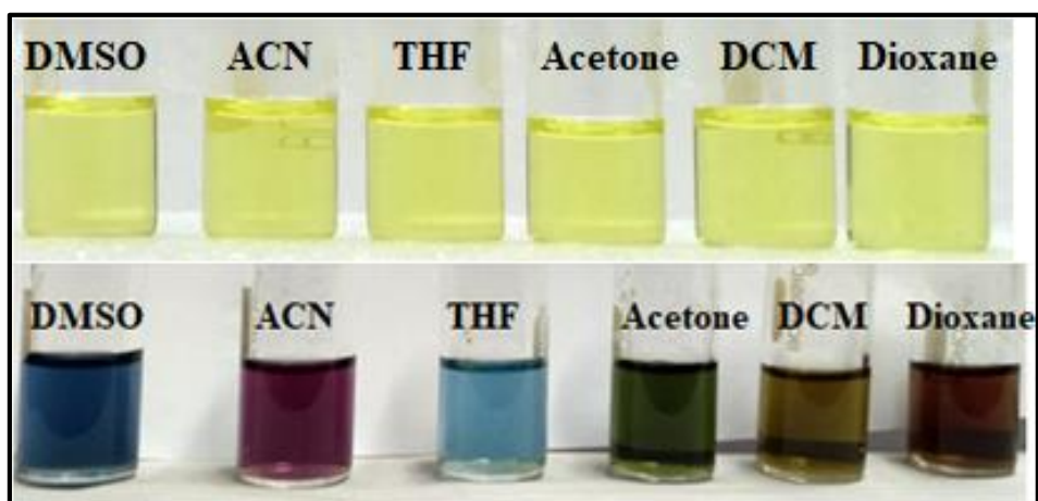
Fig. 4.44 Solvatochromic effect upon addition of 2 equiv. AcO - ( 1 \times 10^{-2} M in DMSO) to the L3R2 ( 1 \times 10^{-5} M) solution in various solvents with different polarities
