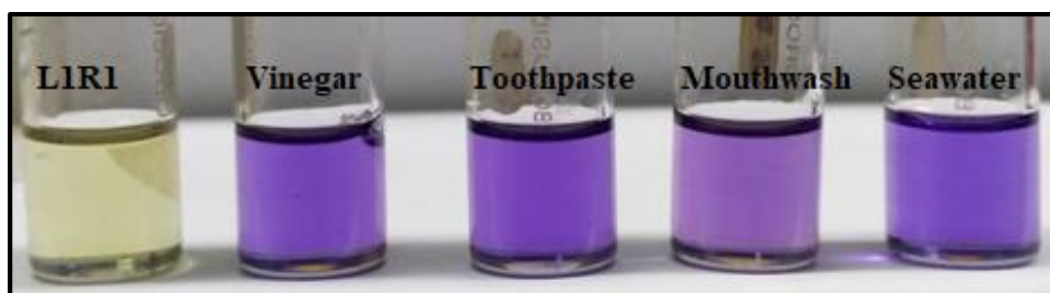
Fig. 2.51 Colour change of the receptor L1R1 ( 4.5 \times 10^{-5} M) upon addition of vinegar, toothpaste, mouthwash, and seawater,
