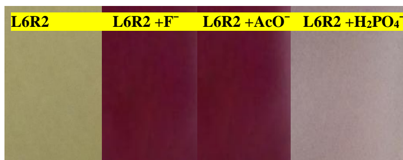
Fig. 7.80 Color changes observed on addition of TBA salts of F^- , AcO^- , and H_2PO_4^- anion to test strips coated with the receptor L6R2 solution
