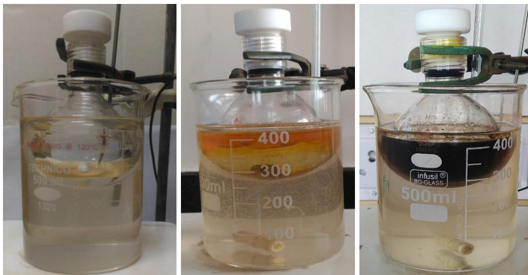
Figure 3.4 Preparation of CMF in a closed batch reactor; snapshots were taken after 5 min (left), 30 min (middle), and 1 h (right).
