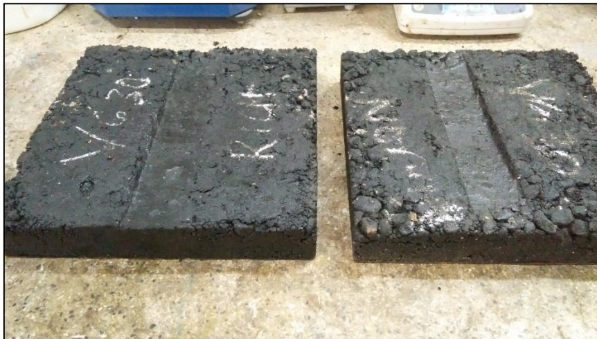
Fig. 3.12 Rutting Specimens after Test
