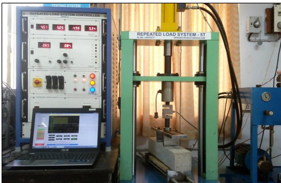
Fig. 3.18 Repeated Load Testing Machine
