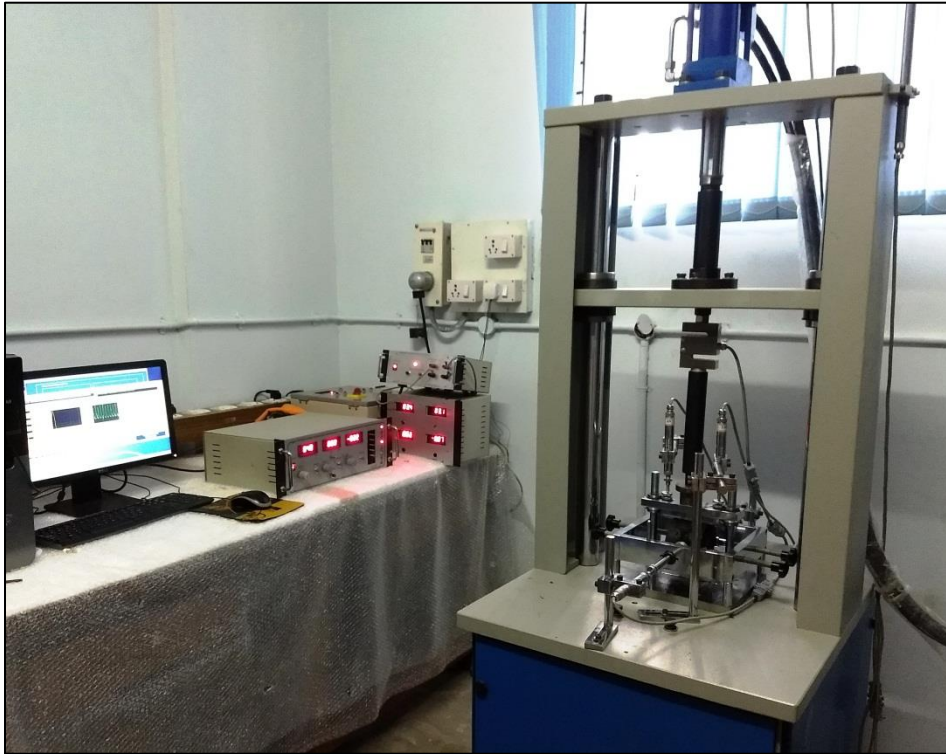
Fig. 3.15 Repeated Load Testing Machine
