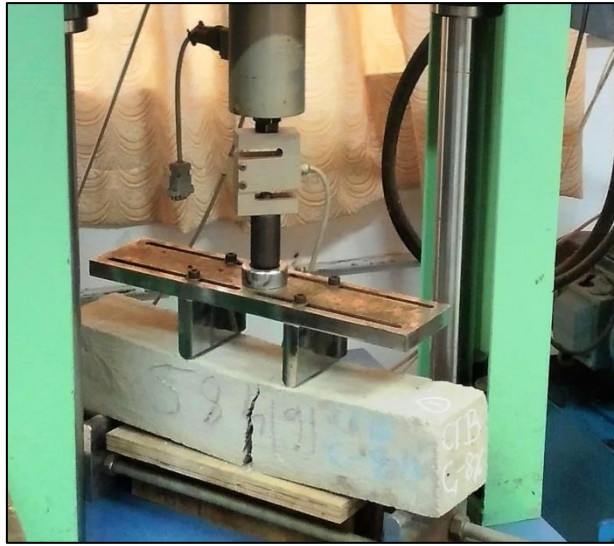
Fig. 3.19 Failed CTA Specimen after Test
