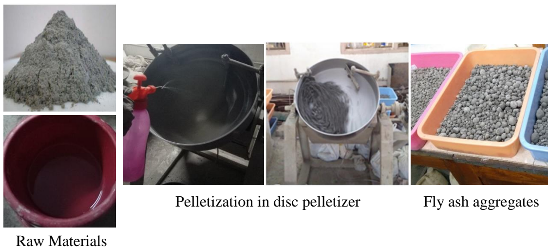
Figure 3.3: Production of fly ash based coarse aggregates using disc pelletizer.
