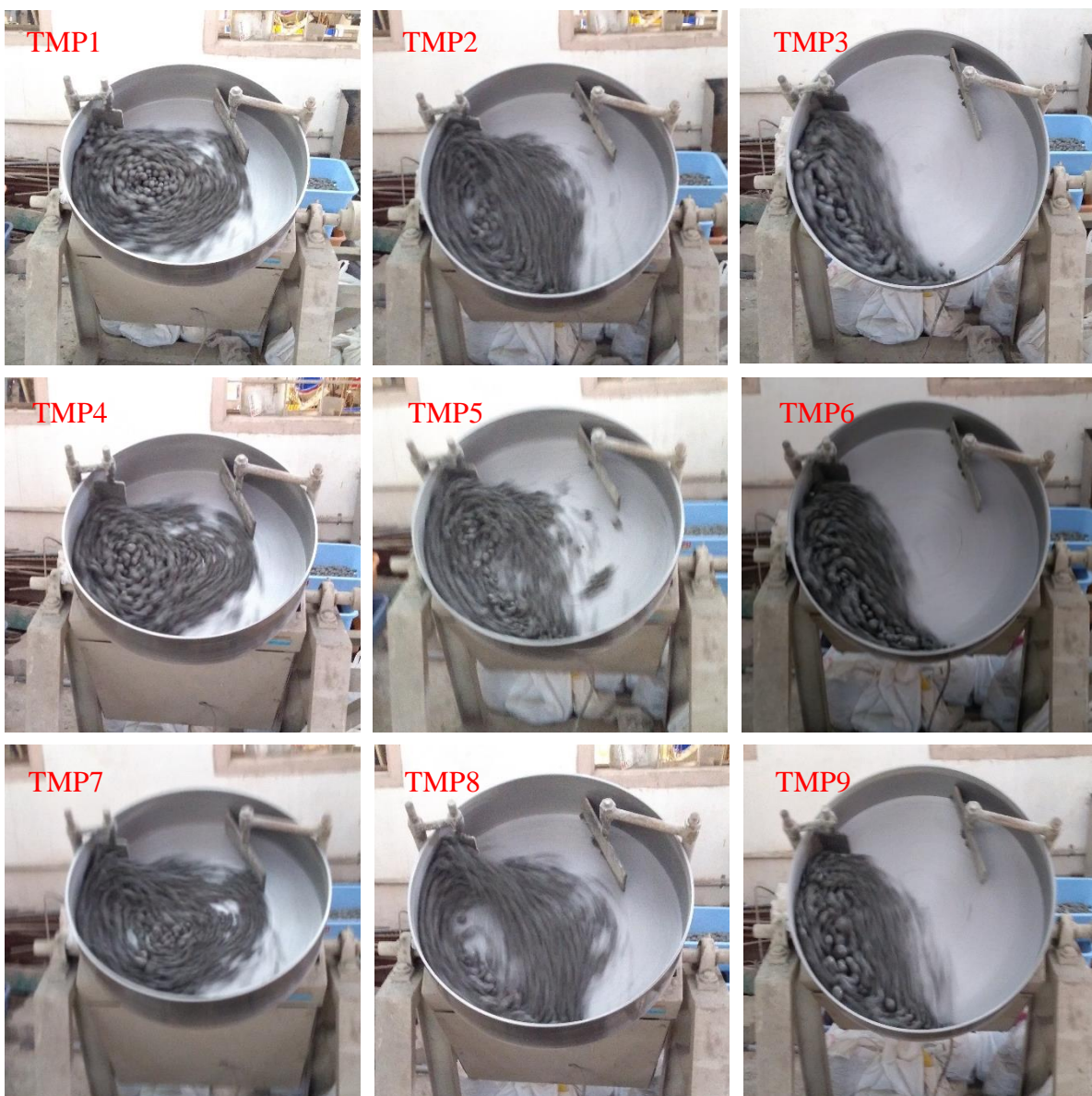
Figure 5.8: Movement of materials at the final stage of pelletization process
