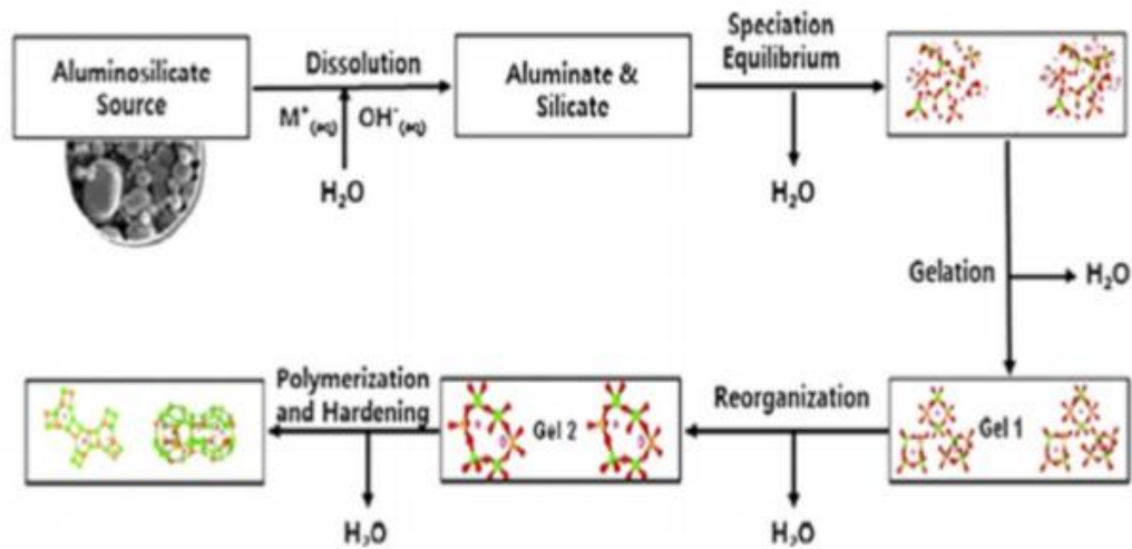
Figure 2.3: Conceptual model for geopolymerisation (Source: Duxson et al. 2007)
