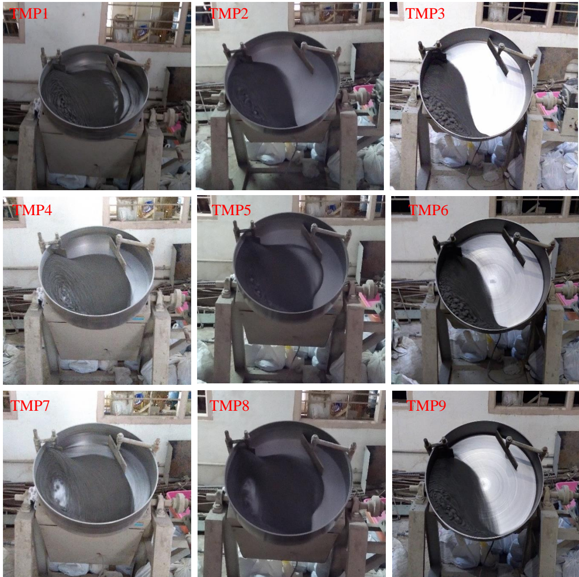
Figure 5.7: Movement of materials at the initial stage of pelletization process
