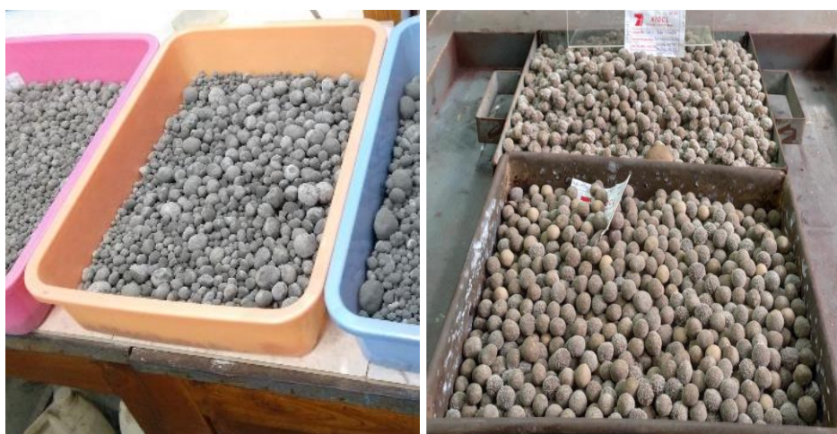
Figure 5.16: Laboratory scale and industrial scale produced fly ash based coarse aggregates
