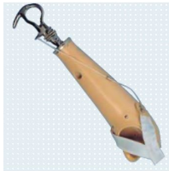
Figure 1.4: Body powered prosthetic hand (Source: (Geethanjali, 2016))
