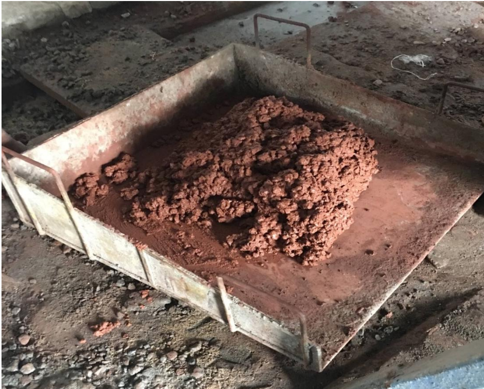
Fig. 3.8 Illustration for concrete mix with Iron Ore Tailings (IOT)-alccofine
