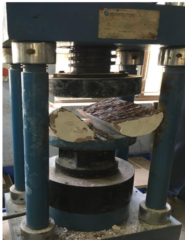
Fig. 3.14 Splitting tensile test on cylindrical sample
