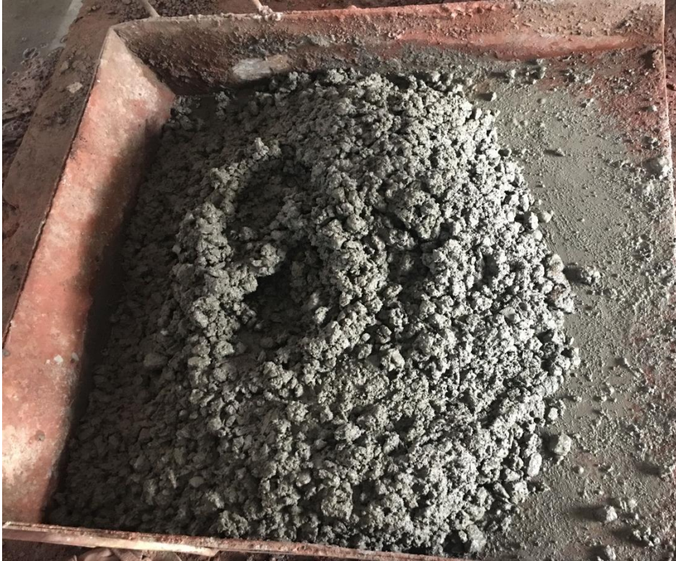
Fig. 3.5 Illustration for concrete mix with Waste Rock (WR) -alccofine
