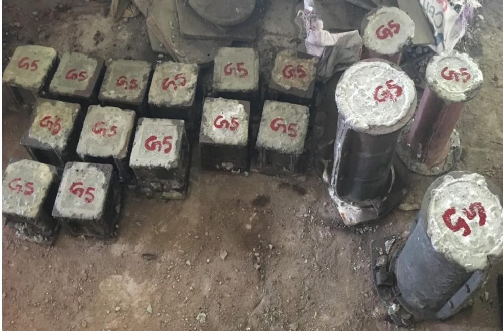
Fig. 3.7 Concrete mix casting with Waste Rock (WR)-alccofine in cubes and cylinder moulds
