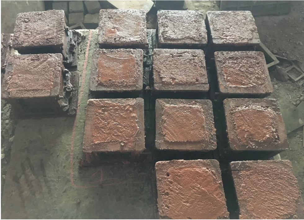
Fig. 3.9 Concrete mix casting with Iron Ore Tailings (IOT)-alccofine in cube moulds
