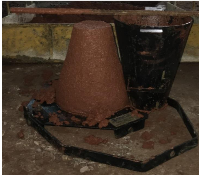
Fig. 3.10 Slump test on Iron Ore Tailings (IOT) concrete
