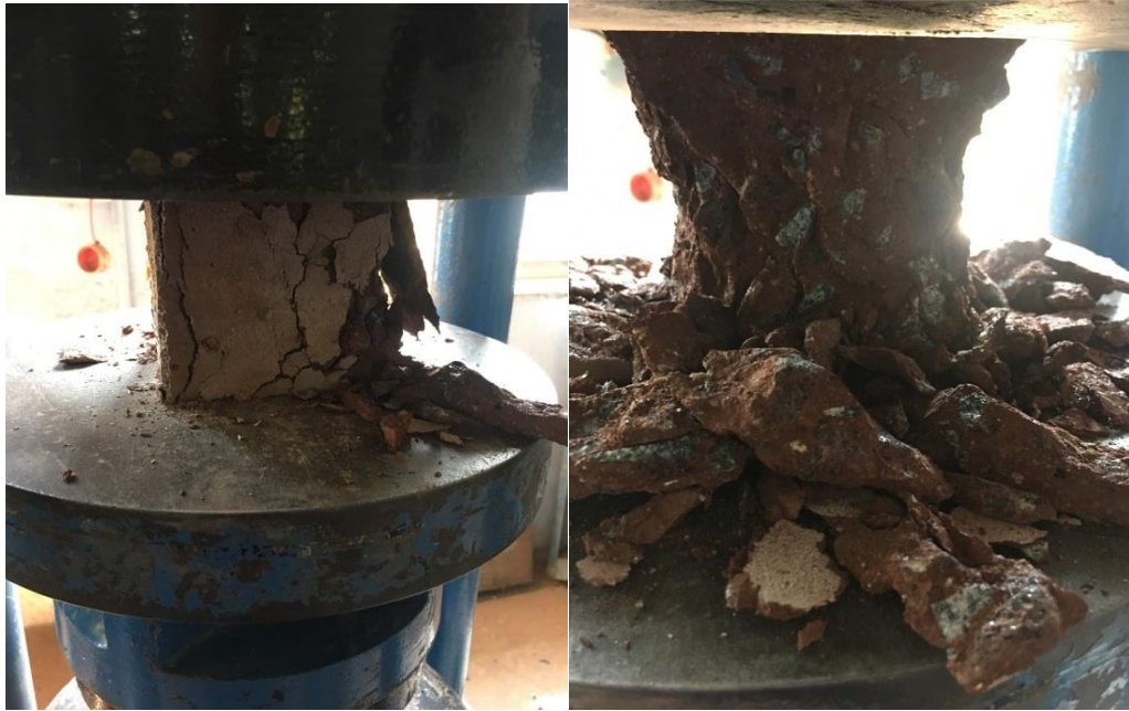
Fig. 3.11 Illustration of compression test on concrete cubes
