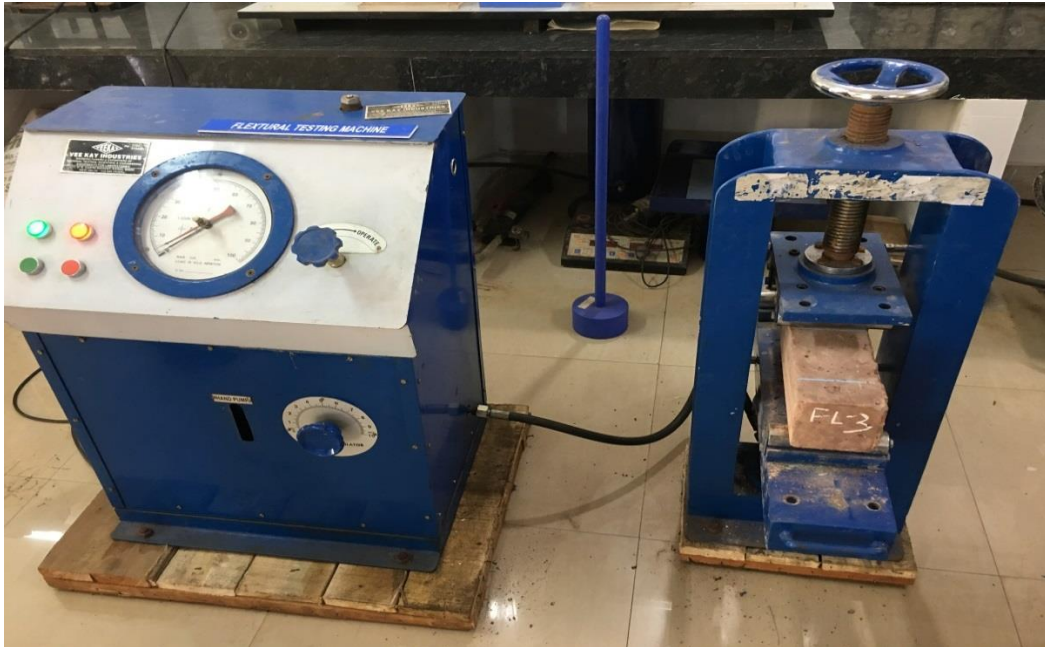
Fig. 3.12 Flexural testing of beam
