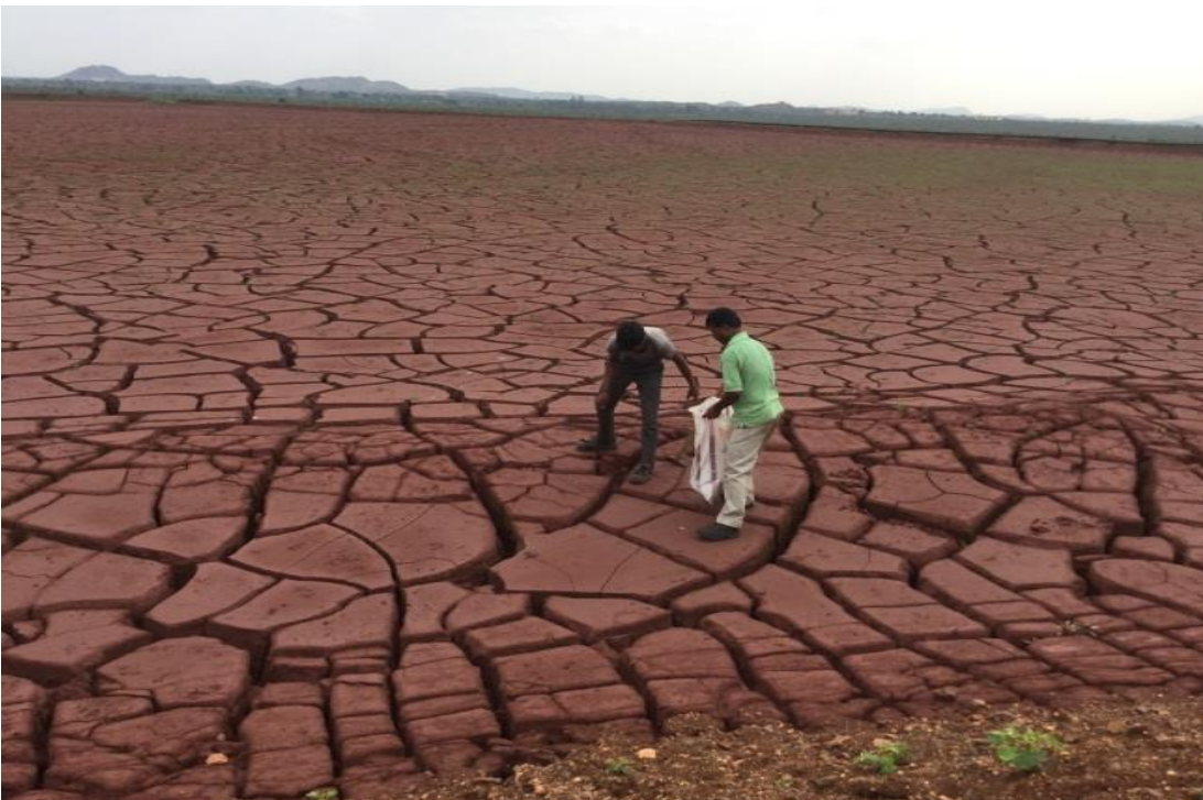
Fig. 3.2 Collection of iron ore tailings (IOT) from tailings pond
