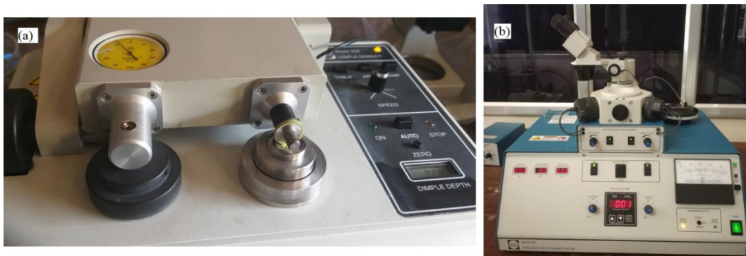
Figure 3.12 Sample preparation for TEM (a) dimpling machine and (b) Ion beam milling machine
