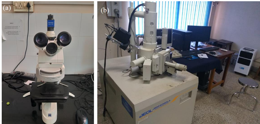
Figure 3.11 (a) Optical microscope (Zeiss, Axiolab A1), (b) Scanning electron microscope (JEOL JSM- 7100F)
