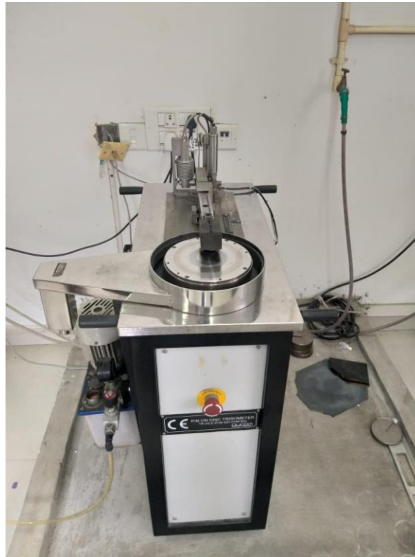
Figure 3.17 Wear testing machine (Pin on disc Tribometer, Ducom)
