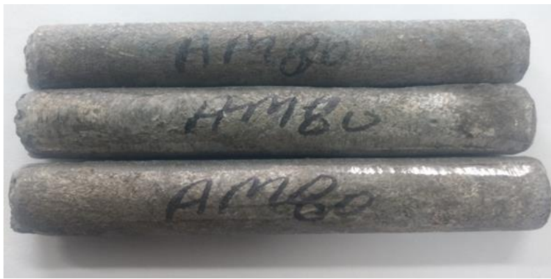
Figure 3.2 Cast AM80 rods in as received condition
