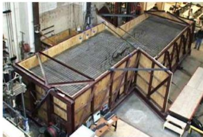
Figure 1.10 Experimental set up to apply strike slip fault to buried pipeline (Lin T. J. et al. , 2012).
