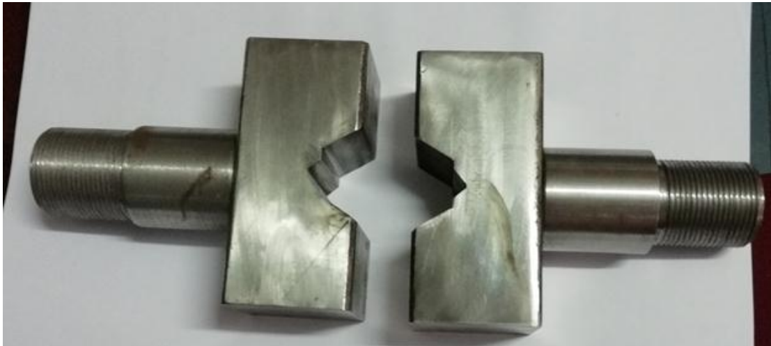
Figure 3.11 Upper end and lower end blocks used to apply axial compressive load to the pipe during the buckling experiment.
