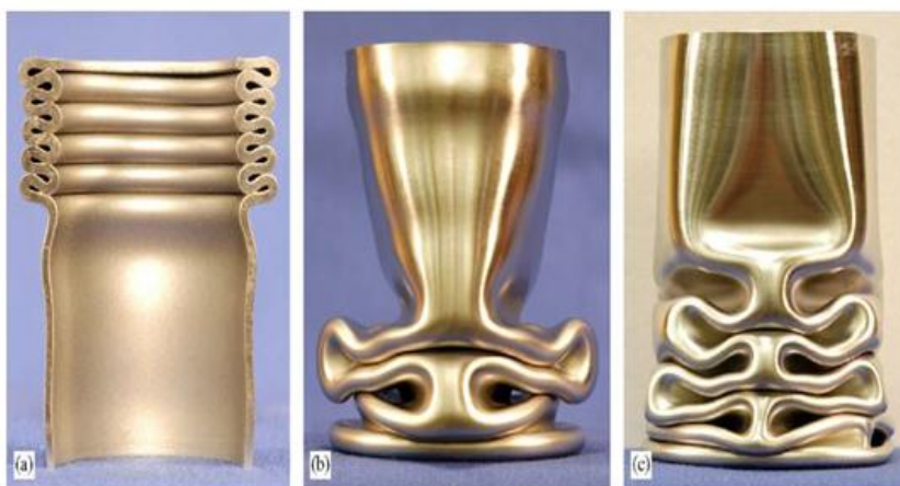
(a) Carbon steel tube that developed axisymmetric concertina folding, (b) mode 2 folding and (c) mode 3 folding of stainless steel tubes.
