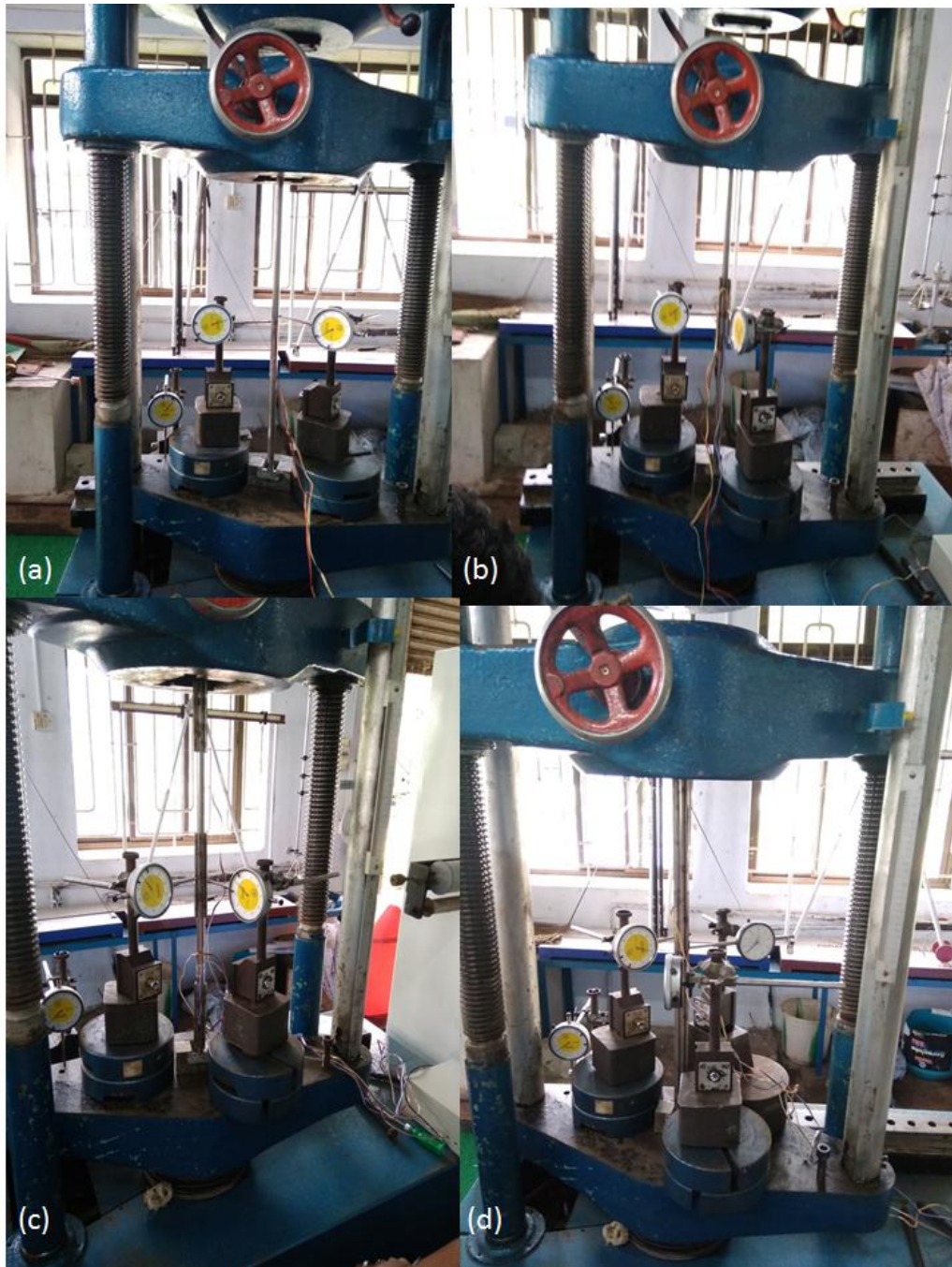
Figure 3.21 Buckling experiments on different pipeline configurations (a) pipeline model without buckle arrestors (b) pipeline model with centrally located buckle arrestors (c) pipeline model with discontinuous buckle arrestors at center and edges (d) pipeline model with continuous buckle arrestors to observe direction of buckling using dial gauges.
