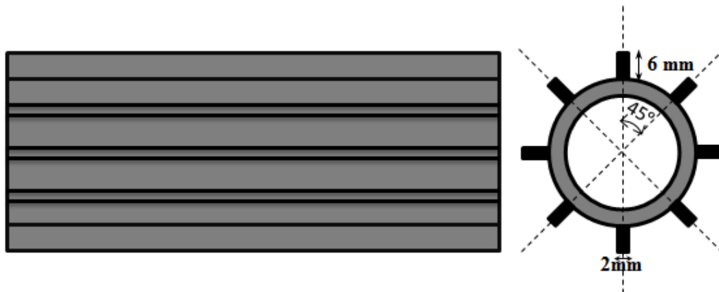
Figure 4.1 Cross-section of longitudinal continuous stiffener model.
