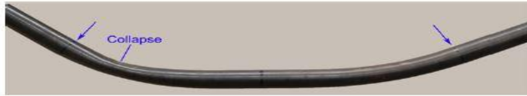
Figure 1.9 Pipe specimen after bending test (Hallai J. F. and Kyriakides S., 2011).
