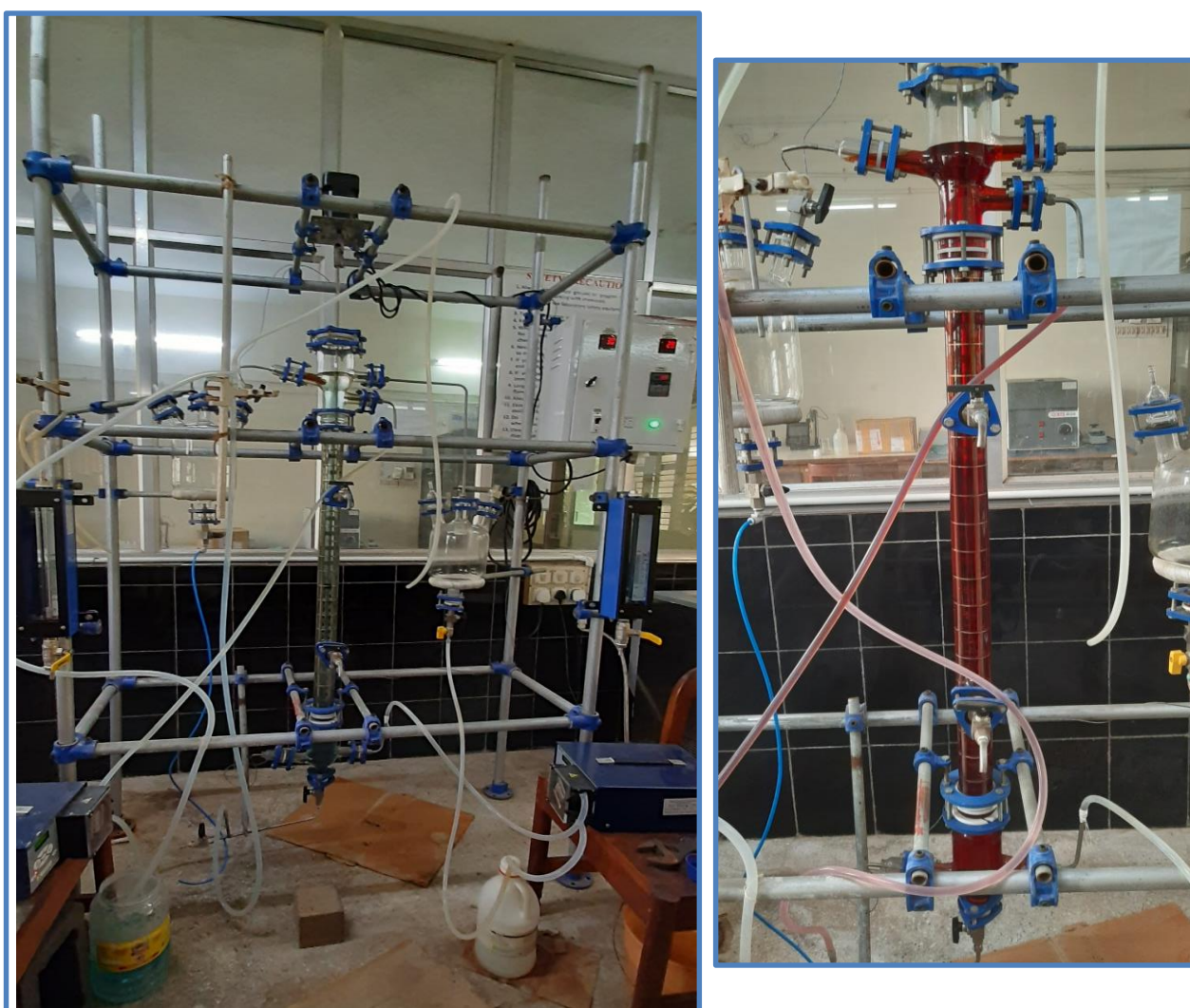
Figure 4.29 The experimental RDC setup in the laboratory for ATP extraction studies
