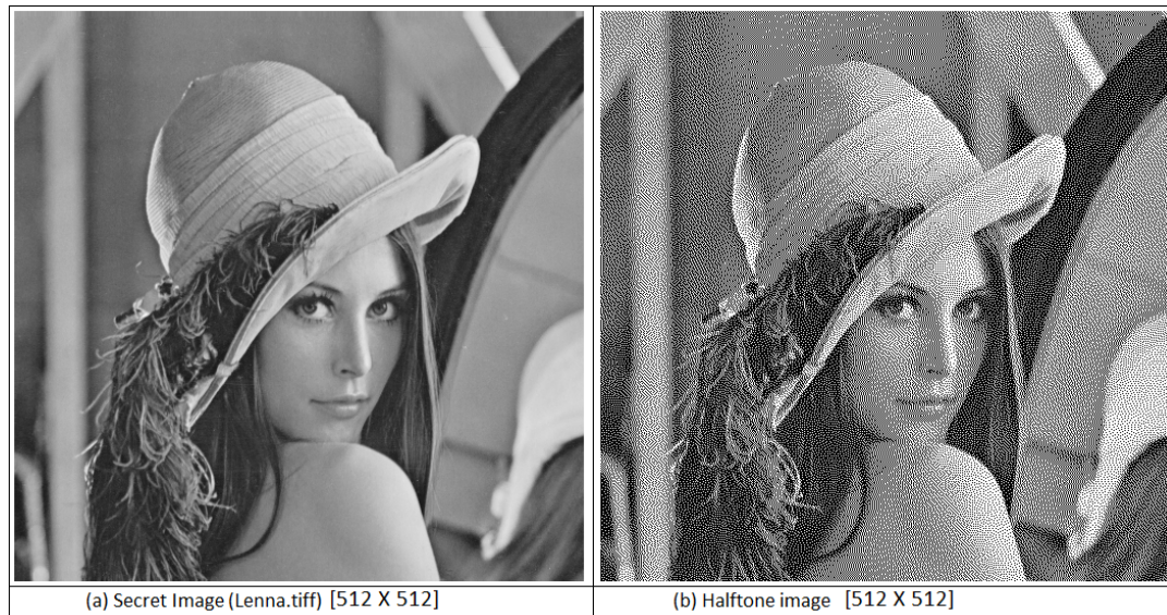
Figure 4.2: The sample input images used : (a) the secret image (lenna.tiff) ( \mathbf{SI} ) (b) Halftone image generated from secret image ( \mathbf{SI}_{halftone} )
