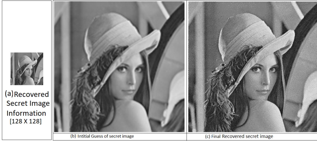
Figure 4.6: (a) Recovered secret image information having size of 128 \times 128 (b) The image used as initial guess to solve SR problem (c) The final restored image having size 512 \times 512 in the gray-scale format
