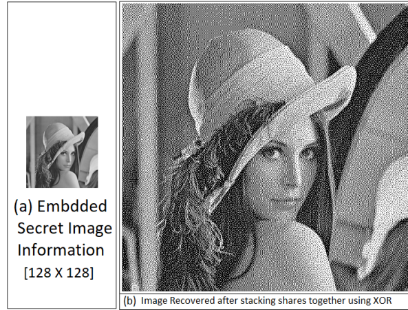
Figure 4.5: (a) The embedded secret image information into the shares (b) The restored image by applying XOR operation on shares ( SI_{xor} )
