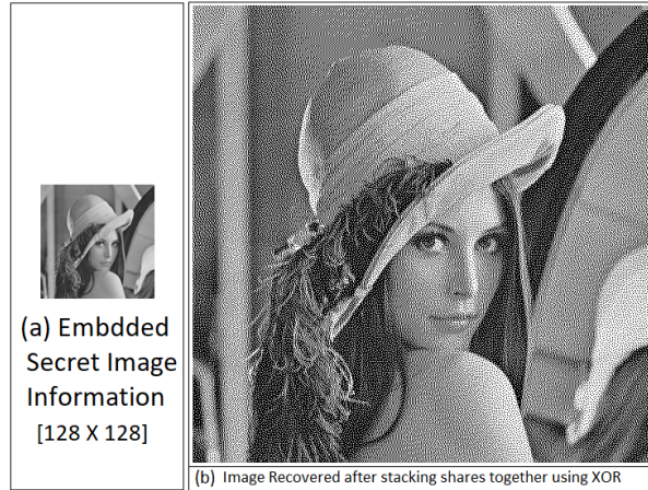
Figure 4.4: (a) The embedded secret image information into the shares (b) The restored image by applying XOR operation on shares ( \mathbf{SI}_{xor} )
