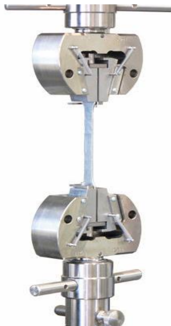
Figure 3.20 Mechanical wedge grippers for clamping tensile test specimen
