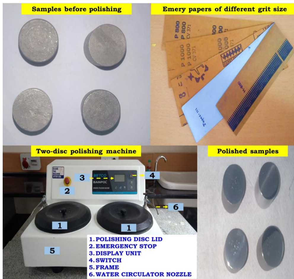
Figure 3.10: Steps involved in sample preparation for metallographic studies.
