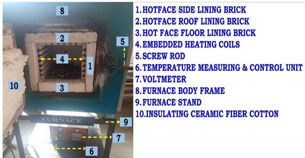
Figure 3.7: Muffle furnace with a temperature controller.
