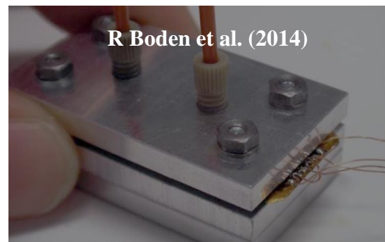
(c) Phase Change actuated micropump
