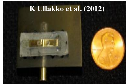
(b) Shape memory alloy actuated micropump
