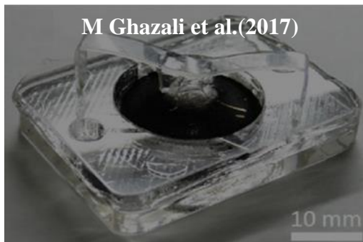
(b) Ionic Conductive Polymer Film actuated micropump
