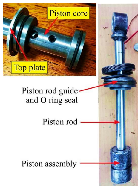
Figure 7.6 Piston assembly with piston rod
