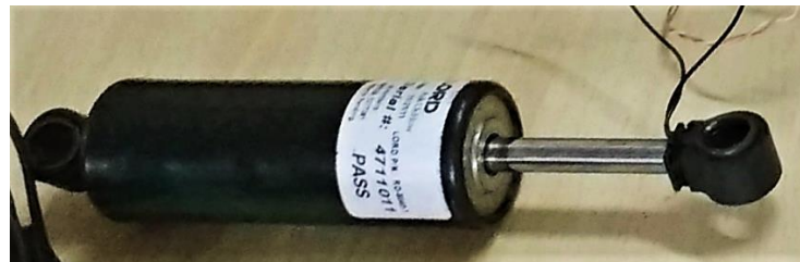
Figure 3.3 Commercial MR damper Lord RD-8040-1
