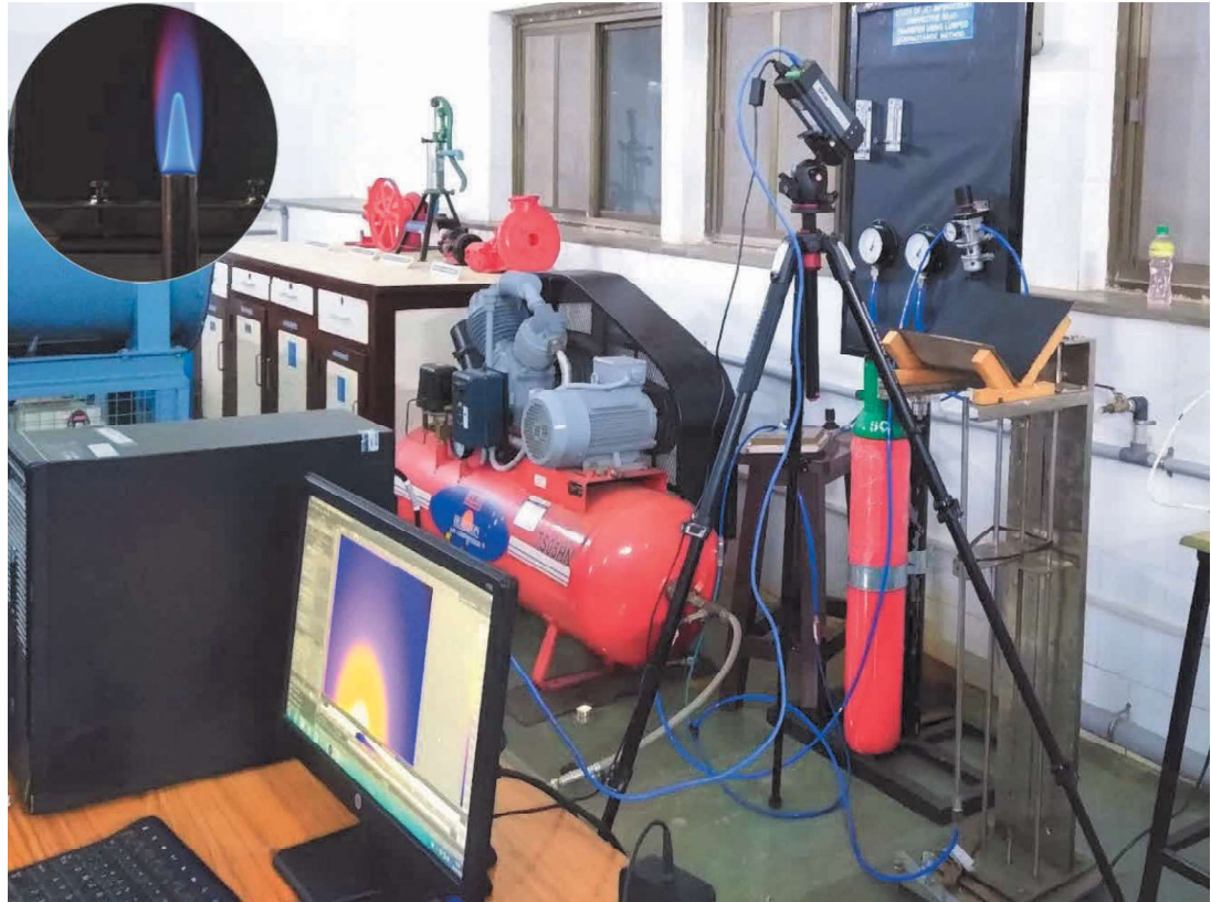
Figure 4.14 Laboratory experimental setup for the study of flame jet impingement over the wedge-shaped test object.
