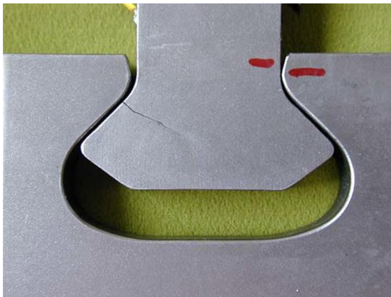
Figure 2.2: Failed turbine blade and disk (Nowell et al., 2006)
