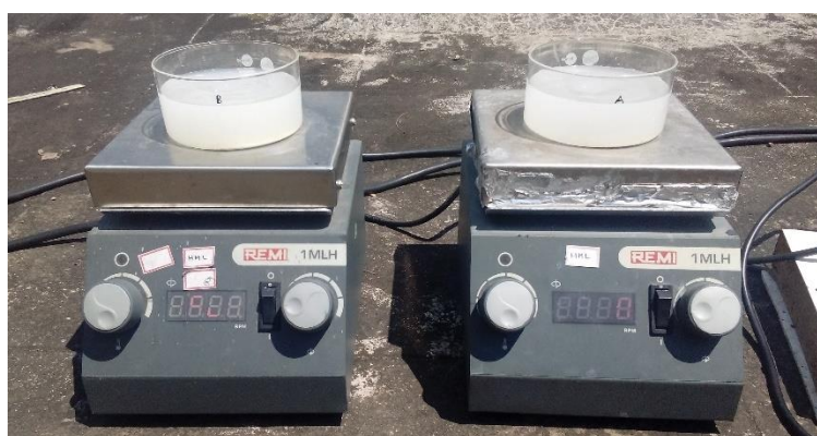
Figure 3.6. Experimental set-up view of batch photocatalytic studies carried out under sunlight
