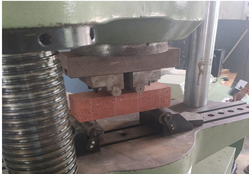
Figure 4.26 Flexural strength test of stabilized ARR
