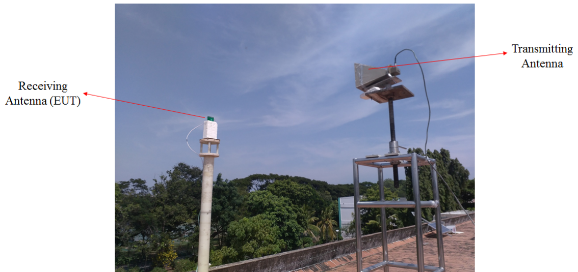
Figure 6.14: Far Field Measurement Setup of Dual Polarized Antenna.
