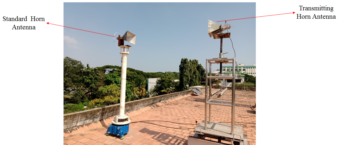
Figure 3.22: Gain Measurement Setup with Standard Gain Horn Antennas .
