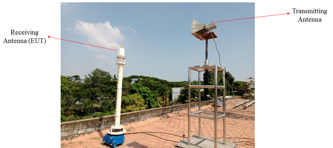
Figure 3.17: Far Field Measurement Setup of Dual Slant Polarized Antenna.
