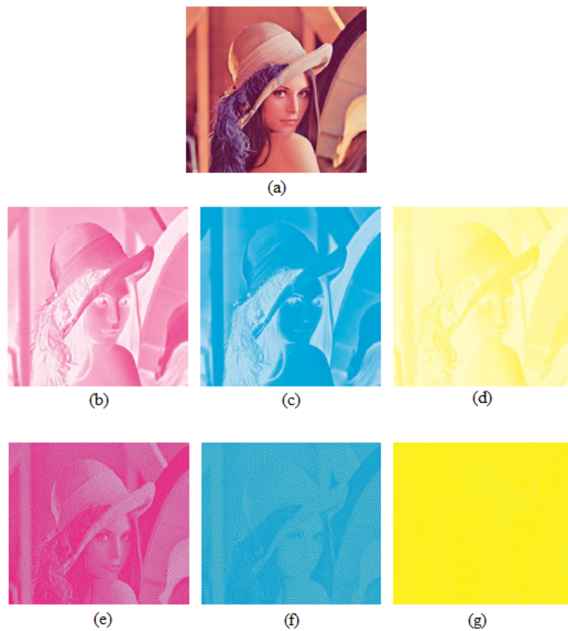
Figure 3.6: (a) Sample colour test image Lenna ( 256 \times 256 ) (b) C component ( 256 \times 256 ) (c) M component ( 256 \times 256 ) (d) Y component ( 256 \times 256 ) (e) Halftone of C component (f) Halftone of M component (g) Halftone of Y component.
