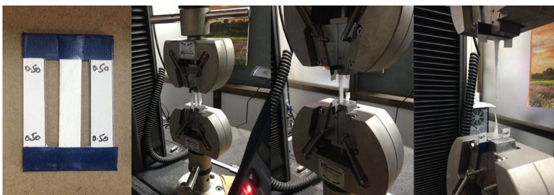
Fig. I.5 Tensile test specimen and testing stages of the talc nanosheets/PVDF nanofabrics.
