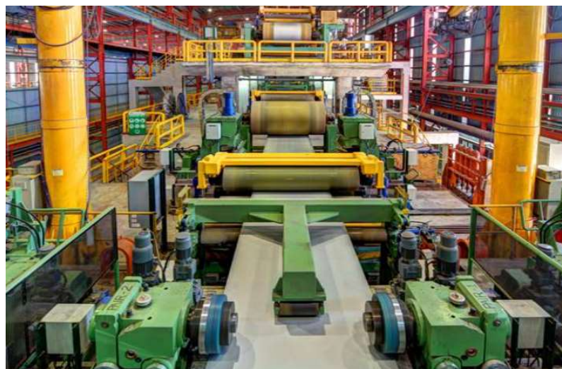
Fig. 5.11. Cold rolling mill line at JSW steel
