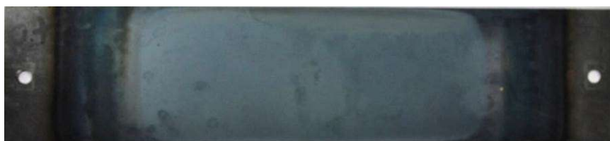
Fig. 4.14. Strip sample after annealing simulation in Gleeble
