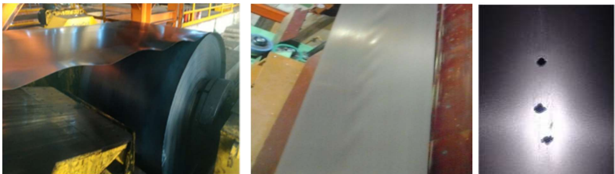
Fig. 1.6. Shape and hole defects in cold rolled IF steels
