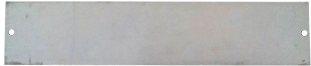
Fig. 1 Specimens for strip annealing simulations in Gleeble
