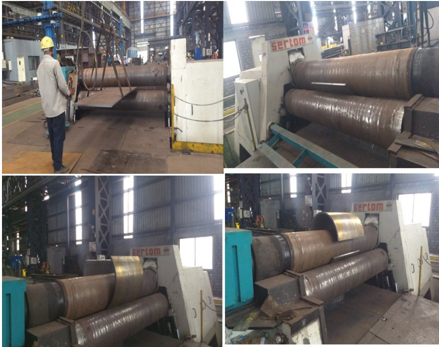
Fig. I.1 Rolling of classifier shell
