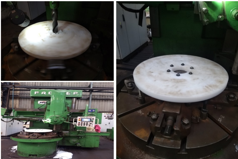
Fig. I.10 Machining of classifier disc
