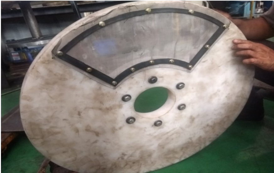
Fig. 4.9 Two dimensional view of classifier disc
