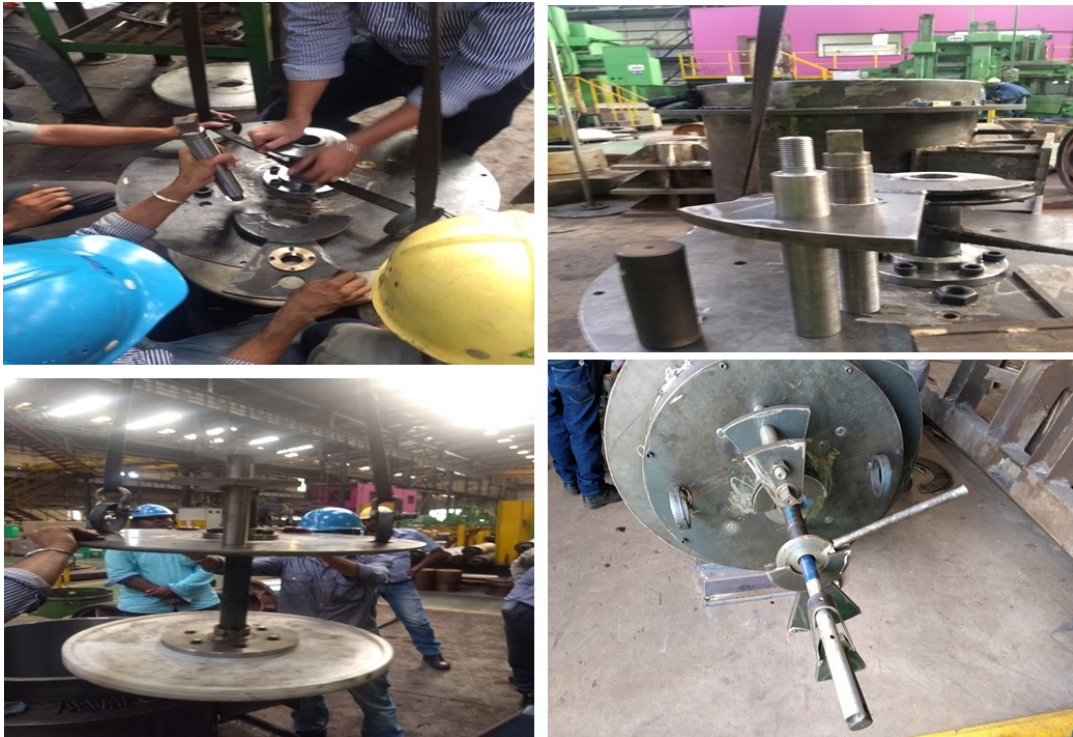
Fig. I.12 Assembly of classifier section
