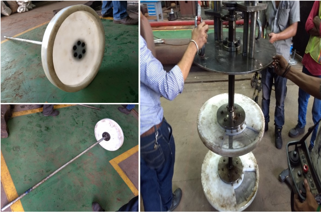
Fig. I.11 Assembly of classifier discs
