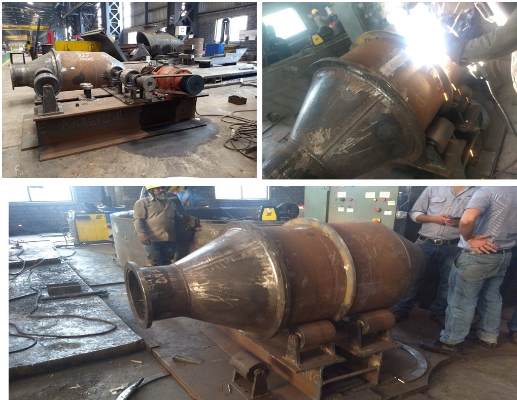
Fig. I.14 Assembly of rotating drum
