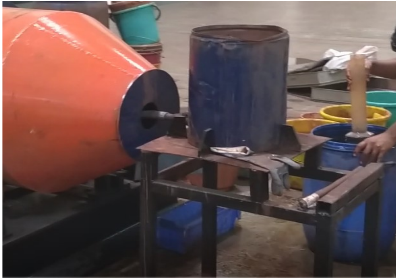
Fig. 4.5 Fabricated feeder arrangement
