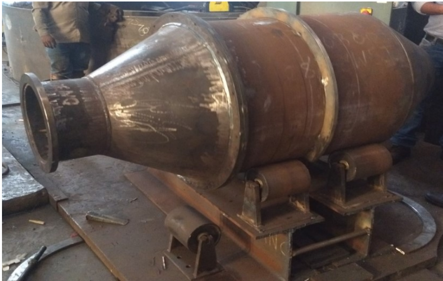
Fig. 4.4 Fabricated grinding shell
