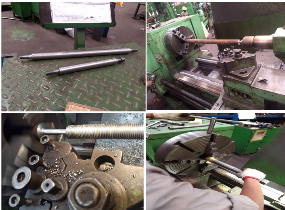
Fig. I.8 Machining of screw and guide rod
