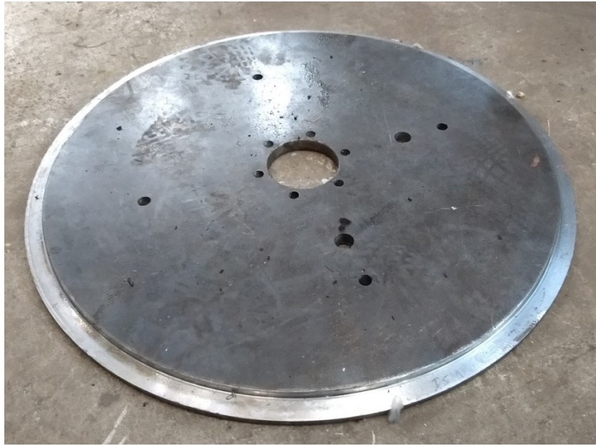
Fig. 4.19 Fabricated classifier closing plate
