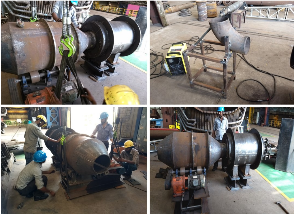
Fig. I.15 Assembly of rotating drum and classifier shell
