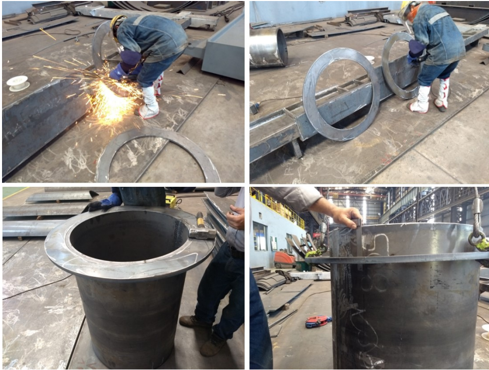
Fig. I.5 Supporting rings for classifier shell
