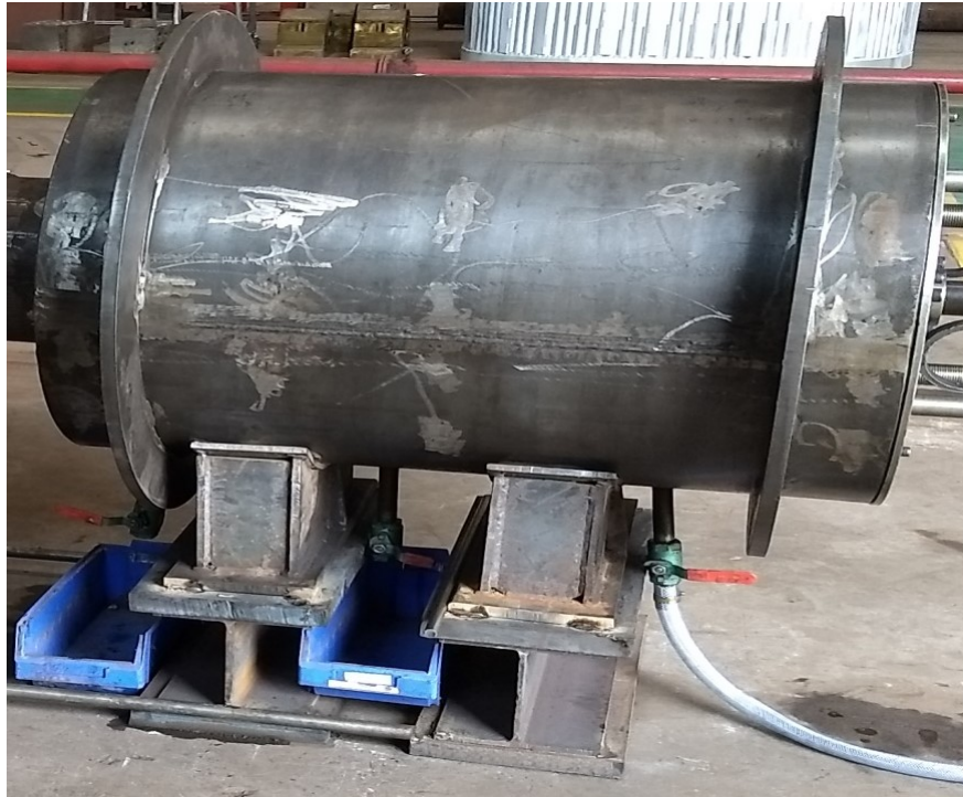
Fig. 4.7 Fabricated classifier section
