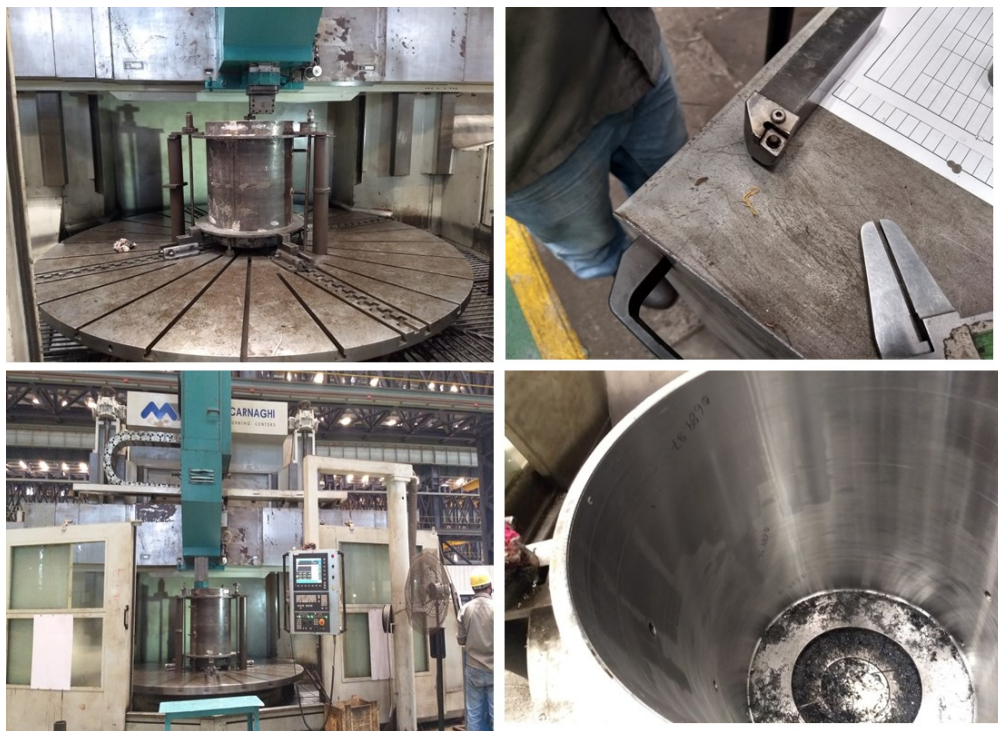
Fig. I.6 Machining of internal surface of classifier shell
