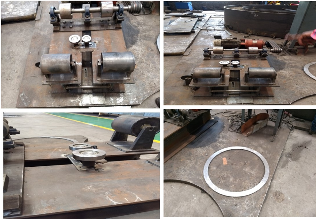
Fig. I.13 Drive system for rotating drum
