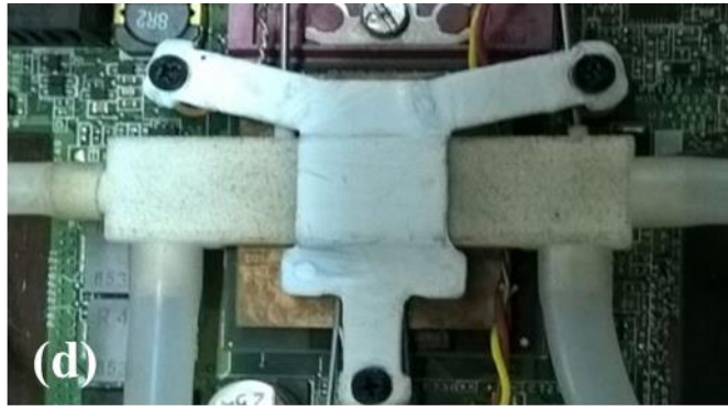
Figure 3.3 Experimental setup of microchannel with heat spreader (a) heat sink, (b) heat sink with FHU, (c) heat sink with sensors, and (d) complete module.
