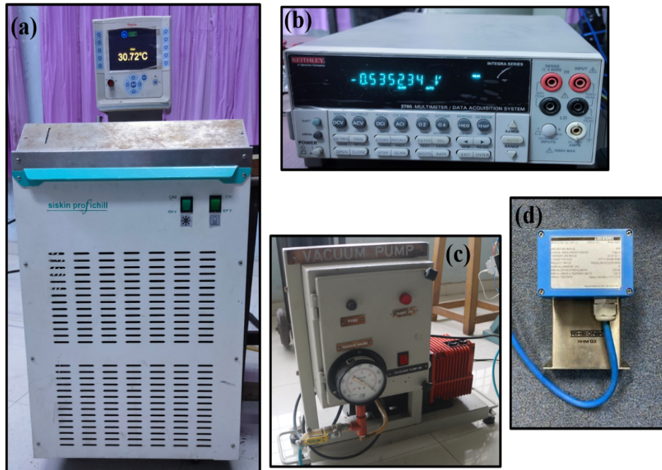
Figure 6.9: Equipment used for test facility (a) Thermostatic bath (b) Data acquisition system (c) Vacuum pump (d) Mass flow meter.
