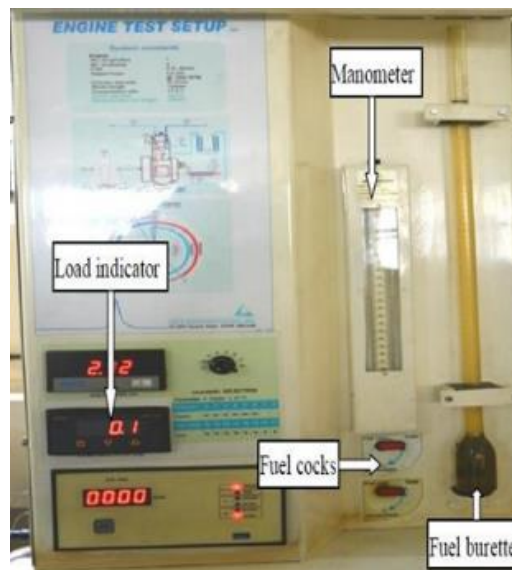
Fig. 3.9 Fuel measurement system
