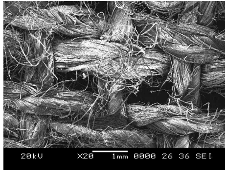
Figure 3.3 SEM image of the flax fabric woven using 3D braided yarns
