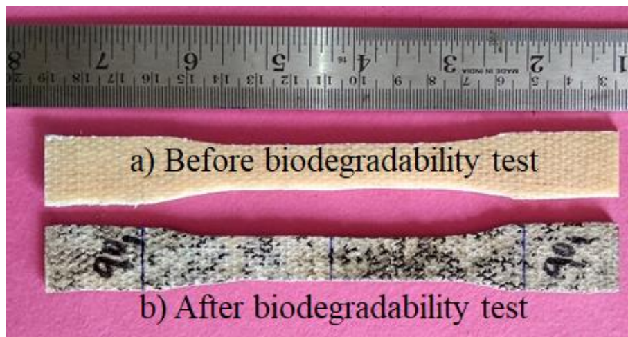
Figure 2.16 Tensile specimens before and after biodegradability test
