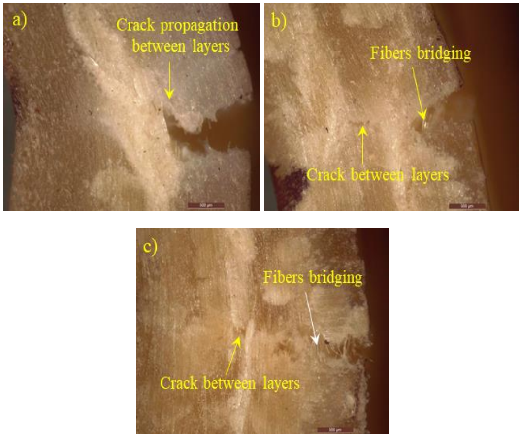
Figure 3.21 Microscopic images of the fractured composite samples from SBS test carried out on a) NFBF11, b) NFBF22 and c) NFBF33 composites
