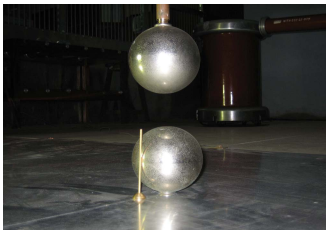
Fig. 1. Sphere gap of 10 cm diameter arranged vertically with electric field perturbing rod in the vicinity. (Both ground sphere and rod are placed on a metallic ground plane).
