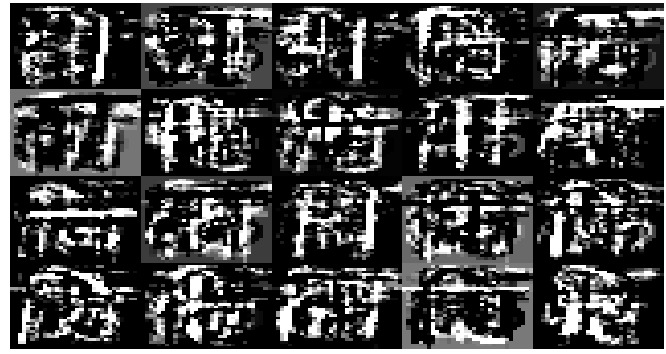
Figure 2. The 20 most significant independent components of the set of font images shown in previous figure.
