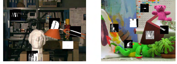
Fig. 3: Support window weight computation on Tsukuba (left) and Teddy (right) images. The weights are computed not only on the active region (which is pure white) but also outside of this region therefore it can cover many variations of intensity value
