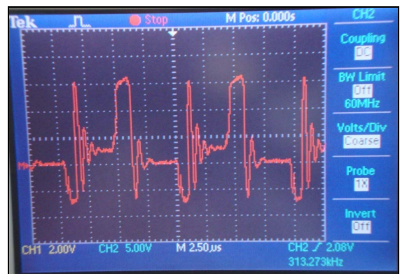
Figure 8. Waveform across the load without snubber circuits
