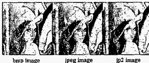
Fig. 4 Comparison of original bmp with JPEG and JPEG2000 compressed images
