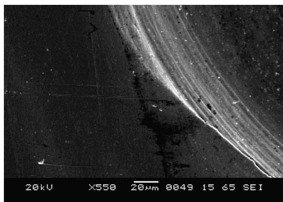
Fig. 5. SEM photomicrograph of sample aged at 500 °C for 2000 h and tested with 12 kg load at 500 °C. Formation of voids in the vicinity of the indentation is seen, but no crack over the grain boundaries.
